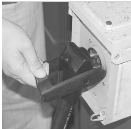
When ready to depart, lift up on handle and pull plug from receptacle
